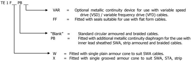
armoured, pliable wire armoured and braided cables. U = Fitted with a universal cone to suit SWA, STA, strip armoured,
